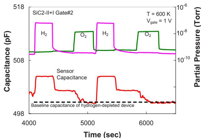
FIG. 5. (Color online) Effect of oxygen on sensor reversibility for a sensor with a nonactivated gate, operated at 327 °C (600 K), 200 K lower than the other measurements reported. When the hydrogen pulse is ended, the capacitance does not return fully to the hydrogen-depleted baseline. For this device at this low temperature, a brief oxygen exposure is required for complete hydrogen depletion.
